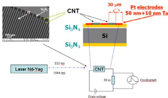
**Figure 1:** The CNT device realized. A Q-Switched Nd-YAG laser is used as exciting source.
